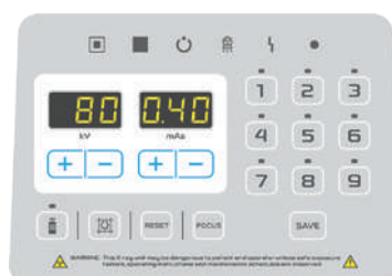
External Operator Control Panel
